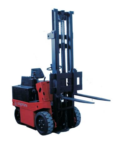
The shown electric truck 1,6 t is one of the versions made with adjustable induction drives – traction and pump one. New decisions are applied at the servo operation also where a hydro motor is used that is CAPRONI JSC production which together with a reducer drives the powerful implementing control mechanisms.
