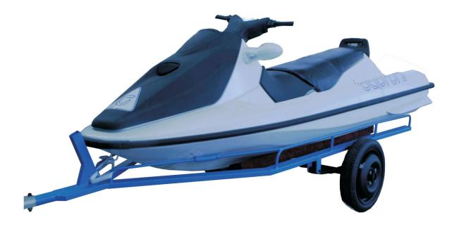
This is Caproni Jsc first attempt for an integrated electric drive in base model jet from the type of Bombardier. The goal is realization of green recreational water vehicle without noise and exhaust good for transport, leisure and sport. Reaching the characteristics of the original jet with internal – combustion engine is NOT a goal.
